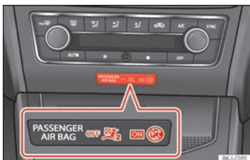
Fig. 28 Centre of the instrument cluster: control lamp for deactivated front passenger airbag in centre console.
