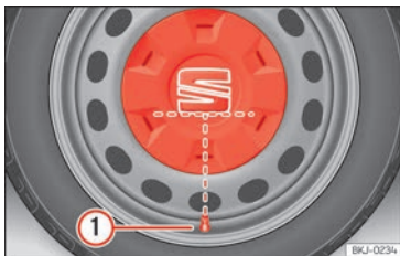
Fig. 182 Correct positioning of the central wheel trim for steel rims.
