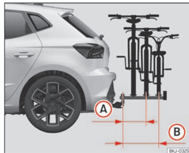
Fig. 144 Schematic representation of the maximum load overhang of a bicycle rack for two or three bicycles.
