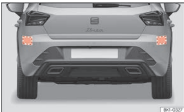
Fig. 97 Rear view of the vehicle: radar sensor areas.
