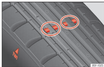
Fig. 179 Tyre profile: tread wear indicators.
