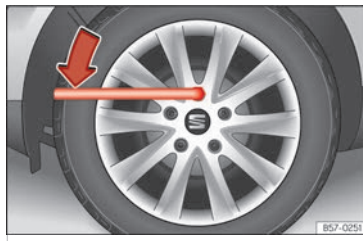
Fig. 186 Tyre change: loosen the wheel nuts.
