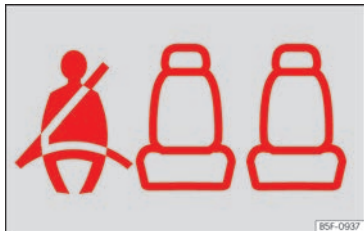
Fig. 18 Instrument cluster: indication of the status of the rear seat seat belts.
