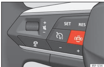
Fig. 93 Left side of the multifunction steering wheel: button for driver assistance systems [depending on the version].
