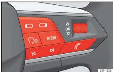
Fig. 10 Right side of multifunction steering wheel: buttons to the menus and informative indications on the instrument panel (depending on the version).
