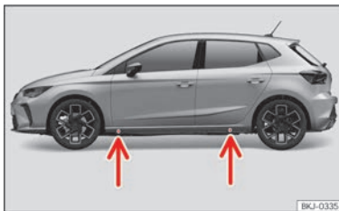
Fig. 188 Jack position points.
