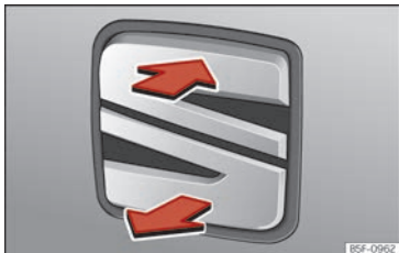
Fig. 55 Rear lid: opening from the outside.
