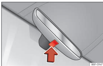
Fig. 77 Manual anti-dazzle function for interior mirror
